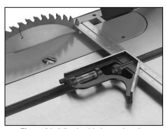
Figure 24. Adjusting blade to miter slot.
